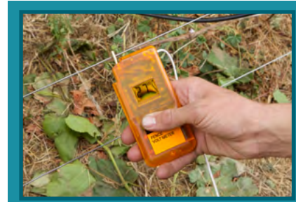
A voltage between 2 and 3 KV is enough to deter beavers.
