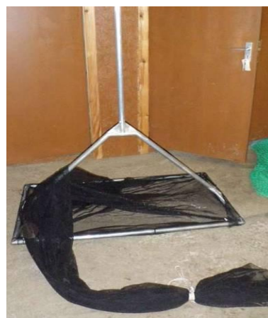
Figures 29 & 30. A specially-designed beaver landing net (SBT). Net frame should be around 100 x 85cm and attached to a ~200cm long iron/aluminium tube. The frame can rectangular or more oval/circle shaped. Joints should be strengthened for durability.
