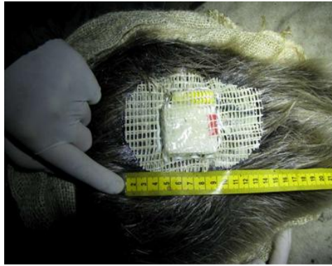
Figure 49. GPS and VHF tag on mesh, glued to adult beaver's back (SBT).
