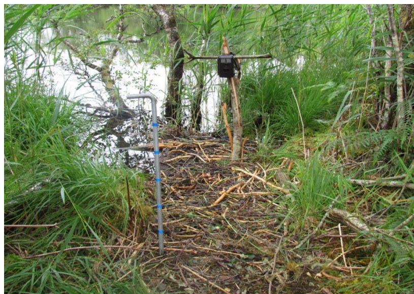
Figure 23. Camera trap located at a beaver feeding station with pole marked in 20cm intervals with reflective tape.
